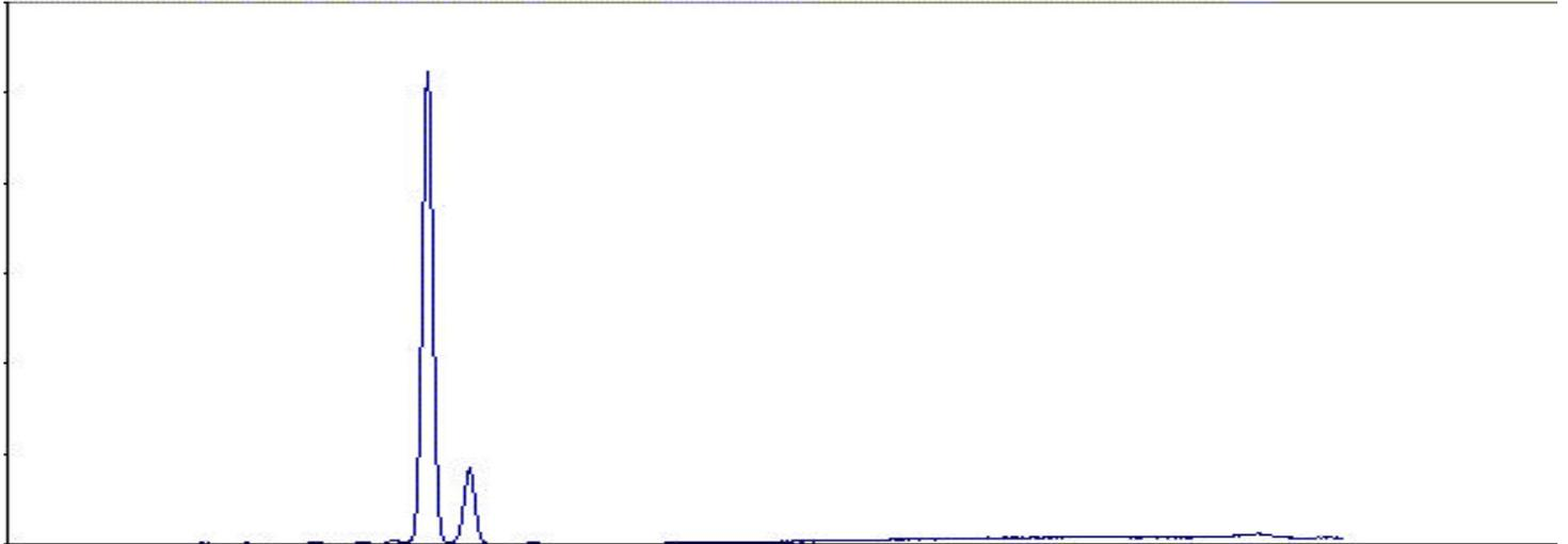
“Finally, I subjected the metallic object to X-Ray Fluorescence (XRF) spectrometry analysis and, as you can see from this spectrum, obtained essentially a pure Fe signal. This is very typical of the spectrum from ordinary carbon steels (the carbon is not detected by this XRF).
